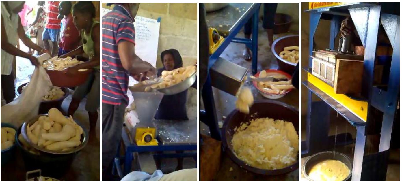
Processing has been improved by installing motor-driven grating mills and liquid-removing presses.
